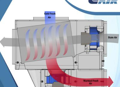
from the outside into the unit where it passes between the aluminum plates absorbing the heat from the exhausting stale air. The clean, dry, fresh pre-heated air is then circulated into the shop. As it becomes stale, it is drawn into the Air Exchanger and the process is repeated.
