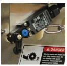
Chain Disk drive units feature an automatic chain tensioning system to reduce maintenance and a safety shut off switch to shut down the system if it becomes plugged by a foreign object.
