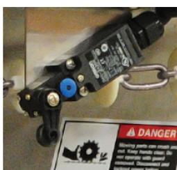
Chain Disk drive units feature an automatic chain tensioning system to reduce maintenance and a safety shut off switch to shut down the system if it becomes plugged by a foreign object.
